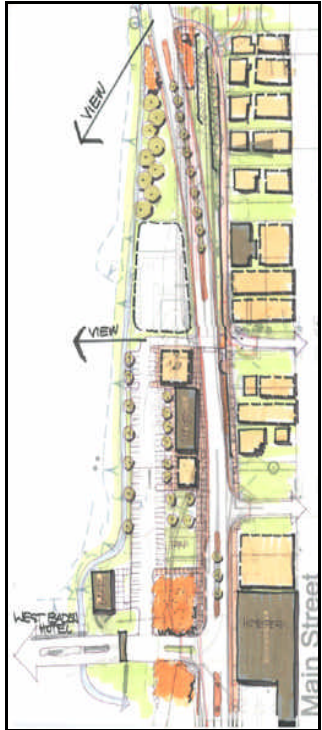
Figure 3.05 – Scarlett Terrace and Hotel Entrance This plan shows how rethinking the road alignment may improve the town and hotel entrance experience, opportunities to rehabilitate Scarlett Terrace and improve walkability of the area.
