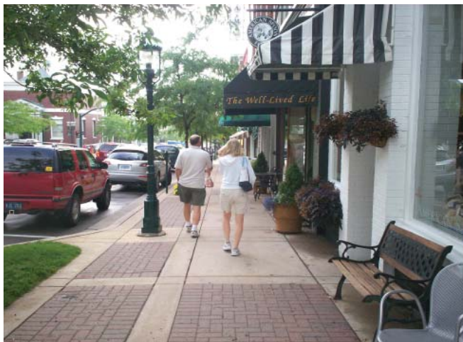
Figure 179.2 A line in the concrete demarcates the frontage zone and provides an organizing element for items such as planters and furniture. The pedestrian way remains clear.
